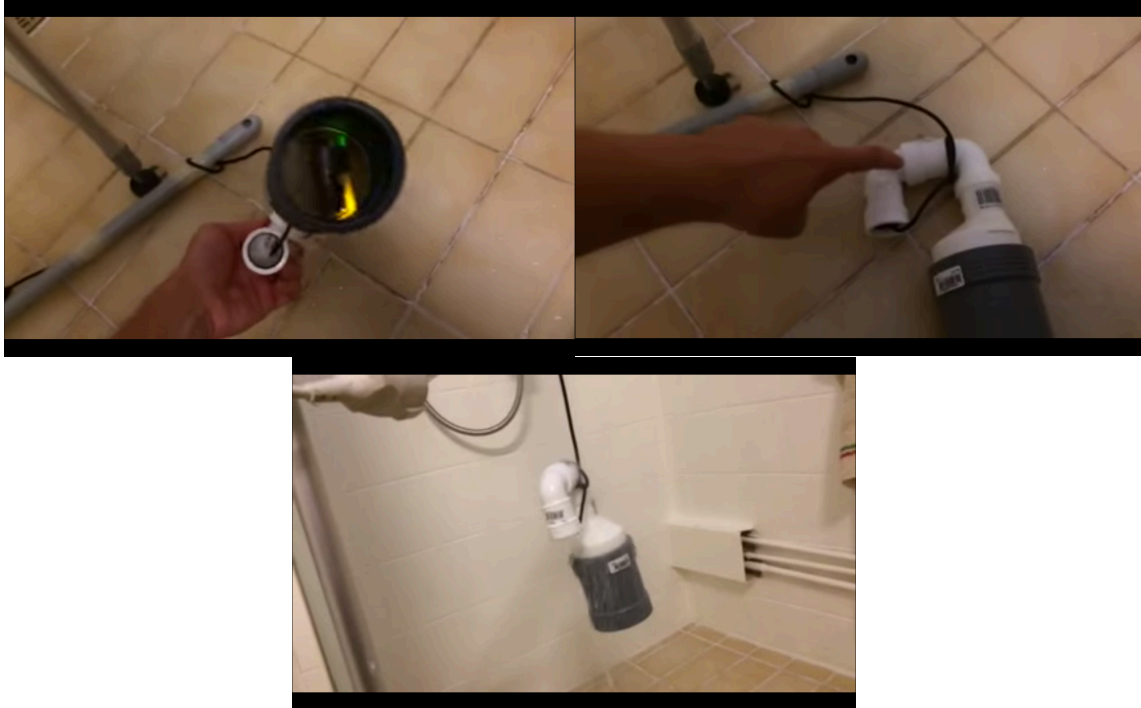
Figure 2 Screenshots showing the prototype of a drain-pipe housing for the Smart Citizen Kit
